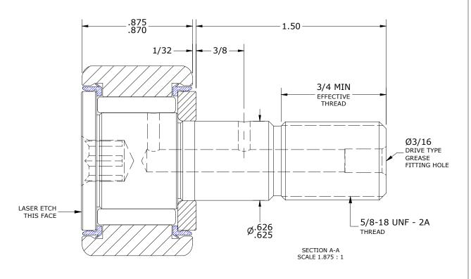
OUTER RING - XD15NW, STAINLESS STEEL, HEAT TREATED STUD - XD15NW, STAINLESS STEEL, ZONE HARDENED WASHER - XD15NW, STAINLESS STEEL, HEAT TREATED NEEDLE ROLLER(S) - XD15NW STAINLESS STEEL, HEAT TREATED SEAL(S) - SYNTHETIC
