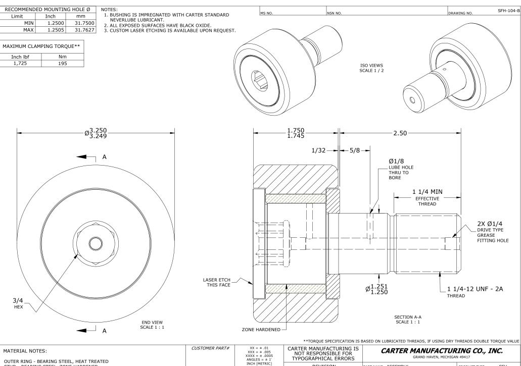
INCH [METRIC] FRACTION = ± 1/32 REVISION PART NAME: ASSEMBLY STUD - BEARING STEEL, ZONE HARDENED PRODUCT TYPE: SFH WASHER - STEEL, HEAT TREATED **E**NGINEERING **C**HANGE **O**RDER NOTE AUTHOR BY DRAWN BY CHK'D BY SALES MATERIAL BUSHING - SINTERED BRONZE В NOTED HG SGW MDNC REVISON BY DATE DATE DATE DATE SHEET SGW 1/5/2021 12/19/2016 1/5/2021 1/5/2021 1 OF 2
