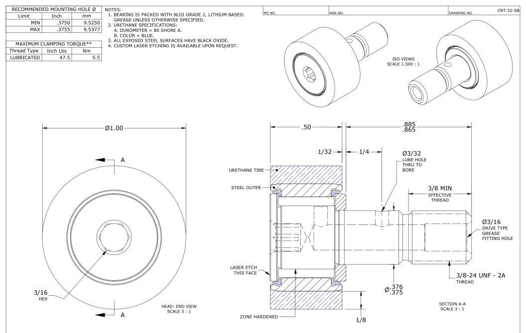
\*\*TORQUE SPECIFICATION IS BASED ON LUBRICATED THREADS, IF USING DRY THREADS DOUBLE TORQUE VALUE
