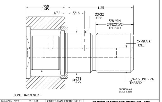
OUTER RACE - BEARING STEEL, HEAT TREATED STUD - BEARING STEEL, ZONE HARDENED NEEDLE ROLLER - BEARING STEEL, HEAT TREATED WASHER - BEARING STEEL, HEAT TREATED\*
