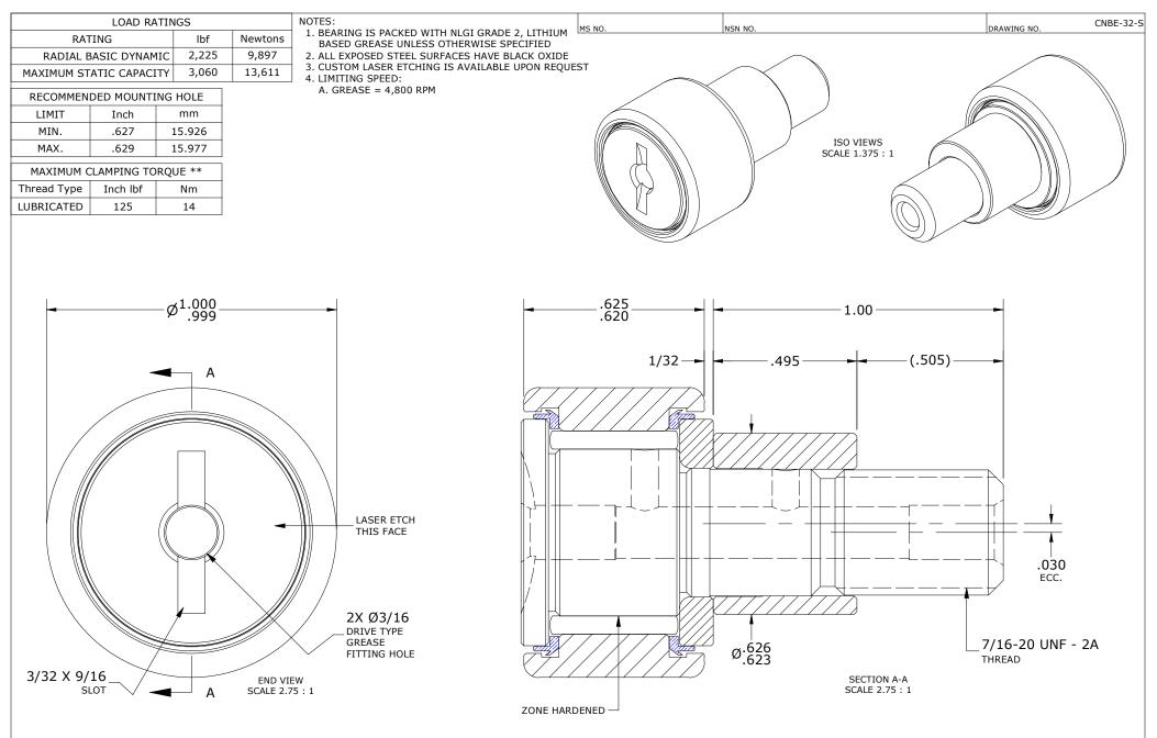
\*\* TORQUE SPECIFICATION IS BASED ON LUBRICATED THREADS, IF USING CLEAN DRY THREADS DOUBLE TORQUE VALUE
