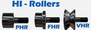
Hi-Rollers are designed for applications where both radial and thrust loading are present. Available with deep groove ball bearings or tapered rollers, they come in v-groove, plain and flanged styles.
